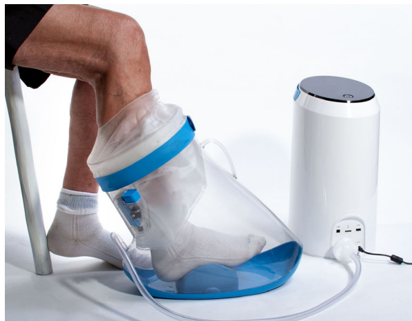
Figure 1. Intermittent negative pressure generated in a pressure chamber sealed around the lower leg, by control unit that is actively removing air from and passively venting the pressure chamber.
